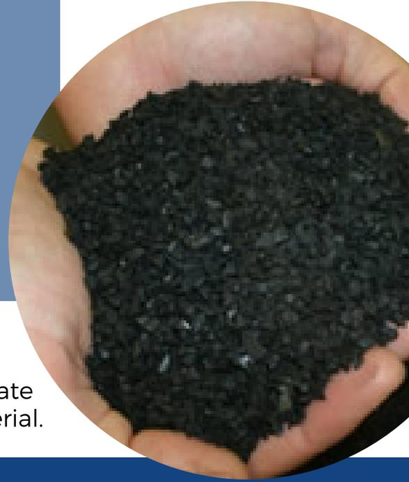
Our Premium Rubber Granules are manufactured from virtually new industrial scrap rubber. The raw material is generated from molding and extrusion processes that create off-spec parts, obsolete inventory, and process waste material.
